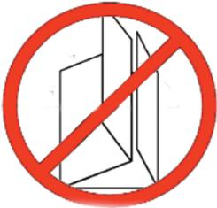
You should avoid creasing, crinkling, folding or standing on your solar panel as this can damage the silicon solar cells and degrade the performance of the solar panel.
