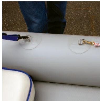
Adjust the clip at the end of the rope-stay and then secure it to the D-Ring on the opposite side located forward of the seat. For kayaks that are not equipped with D-Rings you can secure the clip to the loop on the base of a deluxe inflatable seat.
