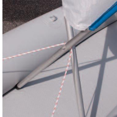
Run the rope-stay around and then through the middle of the frame just below the sail.
