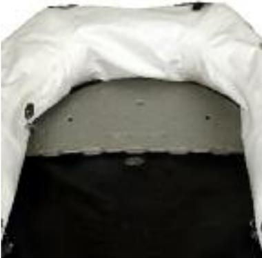
Insert the FB-1 into the bow of the boat. Lift the sides of the boat as necessary in order to slide the FB-1 into place. At this time it does not need to be fully inserted.
