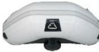
**NOTE:** Inflate the rigid inflatable keel as much as possible with the foot pump until resistance is met. The rigid inflatable keel greatly improves steering performance, the structural strength of the boat and softens the impact of the ride when going through waves.
