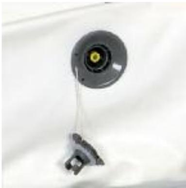
To deflate, remove the cap, press down on the valve stem and turn clockwise to lock into position. Release around 50-75% of the air from each chamber before fully deflating. Excess air can be pushed out as you roll up the boat.
