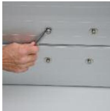
Use the screwdriver at the top of the bolt to hold it in place and at the same time use the crescent wrench on the nuts on the bottom to tighten the bolts for the seat mount.
