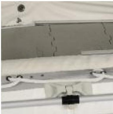
Once deflated, loosen the side stringers with your foot and remove both the stringers and floorboards. You do not need to remove the supports on the FB-2 & FB-4 floorboard pieces. If you have a drop stitch floor, you can deflate it and roll it up with the hull.
