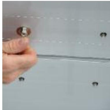
Once the bolts are in you can then install the washer and the bolt on the underside of the seat board where the four bolts stick out.
