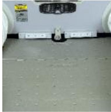
Insert the FB-3 so that it meshes with the FB-4 and overlaps the FB-2. Lift the ends of the FB-2 and FB-3 and connect them to form an inverted V. Apply pressure to the joint to secure the floorboards into place.
