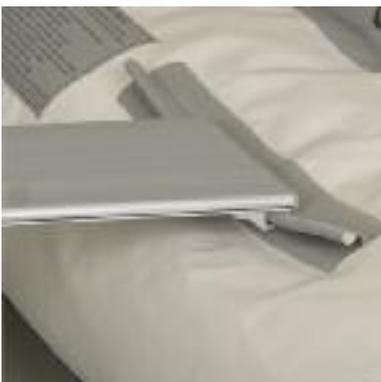
Begin by feeding the fabric beads on the pontoons through the nylon slotted fittings underneath the aluminum bench seat. Slide the seat over the fabric beads so that the seat is toward the center.
