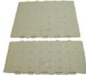
The 14SR features the FB-3 and FB-3 short which are both marked as FB-3. Insert the FB-3 so that it meshes with the FB-4 and overlaps the FB-2 and install the FB-3 short should be installed between the FB-3 and FB-2 floorboards.
