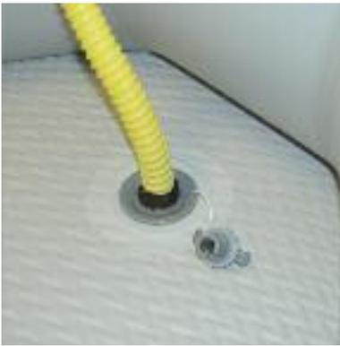
Place the floor inside of the boat with the air valve located in the bow of the boat, facing up. Begin inflating the floor using the high volume setting on the A-50. When resistance is met switch over to the high pressure setting and finish inflating the floor until resistance is met.
