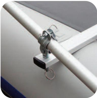
Secure the oar pin underneath the yoke with the ring.
