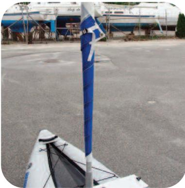
The sail can be furled around the mast without removing the batten. Tightly wrap the sail around the mast. Run the strap through the center of the buckle and out the outer slot. Pull strap tight.
