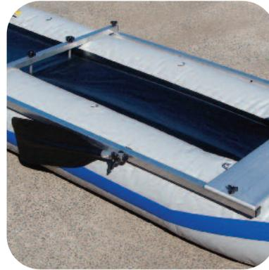
Attach the leeboards to the frame. Place a metal washer on the bolt, put bolt through frame from inside. Place a rubber washer, leeboard, rubber washer, metal washer and butterfly nut on bolt.
