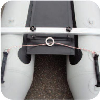
Tie the Sail Ring to the metal rings of the D-ring handles behind the steering yoke.
