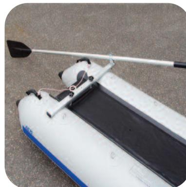
Slide the oar pin onto the handle section of the two-part rudder. Assemble the oar and insert the oar pin into its hole in the yoke.
