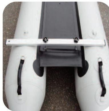
Remove the aft yoke and replace it with the steering yoke provided. The yoke has a hole for the oar pin. The hole can be placed so you can steer right or left handed depending on your preference.
