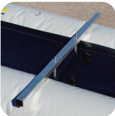
Replace the center yoke bar and bolts with the 36½" tube and the longer (5") bolts included in the kit. If there is vinyl material wrapped around the yoke, remove it now, it is for shipping purposes only.
