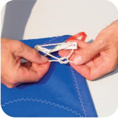
Insert the batten into the opening near the top of the sail. Once it is fully inserted, tie the rope to the fitting.
