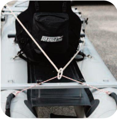
Run the free end of the main sheet through the white ring at the back of the boat and up next to the seat. This rope will control the sail when sailing. You will need to duck your head when tacking.
