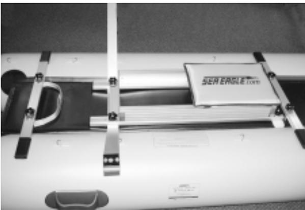
Now snap the collapsible oars together, attach the oarlock pins with bolts and wing nuts. Now drop the oarlock pins in the fittings on the two end of the rowing arm as shown.
